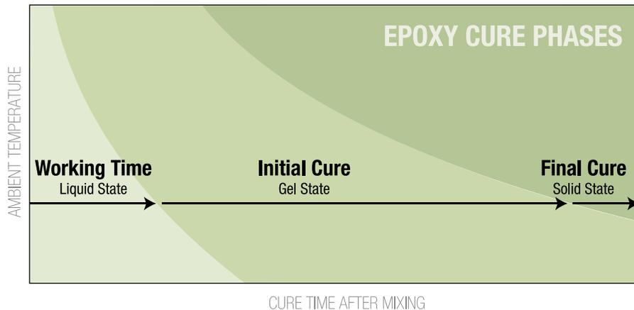
All PRO-SET Epoxies go through the same three phases of cure. The higher the ambient temperature, the shorter each of the phases and overall cure.
