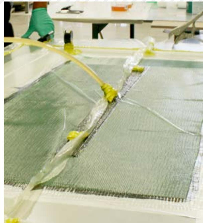
PRO-SET Infusion Epoxies are super low viscosity systems with a range of hardeners to meet the demands of modern infusion processes.
