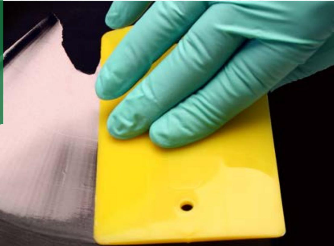
PRO-SET Tooling Epoxy is a 2-part paste formulated for surfacing molds and plugs.
