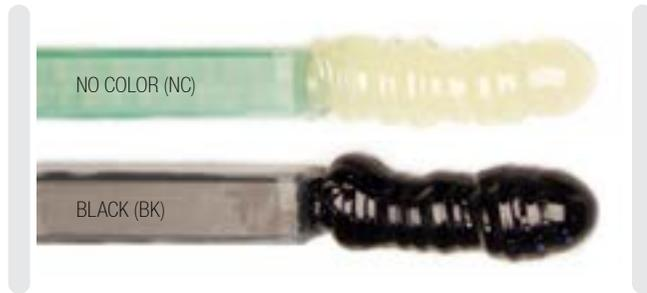
Adhesives based on PRO-SET 175 Resin are paired with Fast (273), Medium (275) or Slow (277) hardener. They are suitable for most composite bonding applications.
